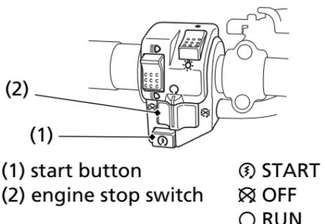
The start button (1) is used for starting the engine. Pushing the button in starts the engine. See *Starting Procedure*, page 48.
