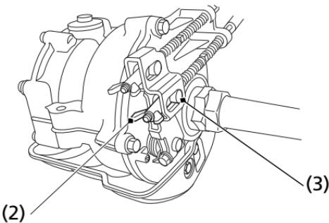
(2) brake pedal adjusting nut
