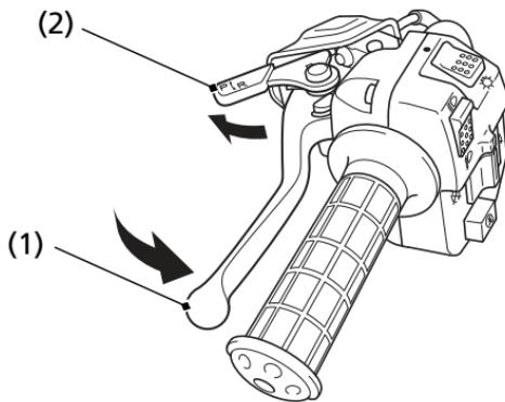
(1) rear brake lever/parking brake lever
