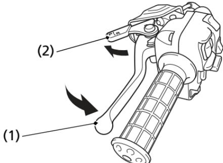
(1) rear brake lever/parking brake lever
