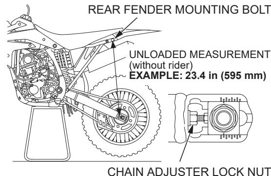
3. Measure the *loaded with rider* dimension. Remove the workstand. With two helpers available, sit as far forward as possible on your CRF's seat, wearing your riding apparel. Ask one helper to steady your CRF perfectly upright so you can put both feet on the pegs. Bounce your weight on the seat a couple of times to help the suspension overcome any situation and settle to a good reference point.
