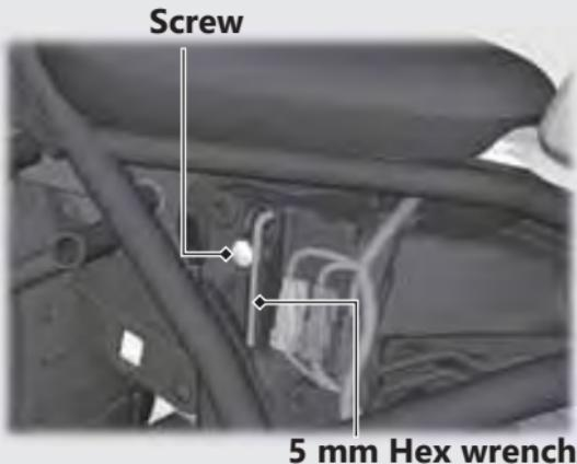
The tool kit is stored on the underside of the seat.
