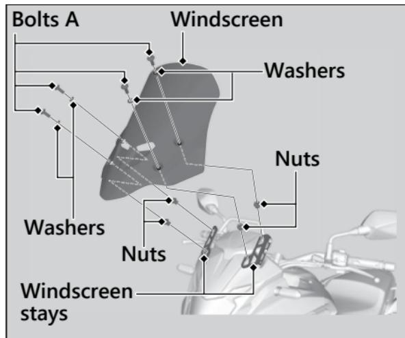
1. Remove the windscreen by removing the bolts A, washers and nuts.
