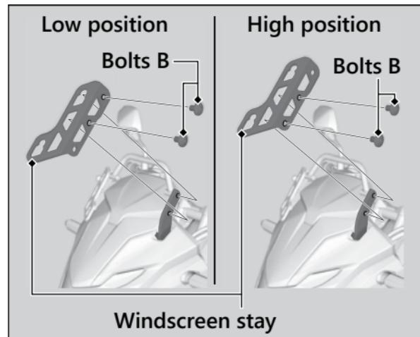
2. Remove the left side windscreen stay by removing the bolts B.
