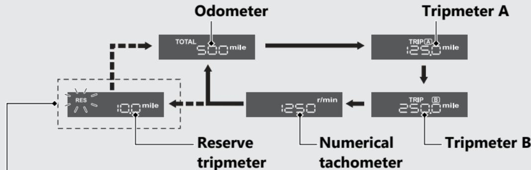
**When the 1st (E) segment of the fuel gauge starts flashing**
