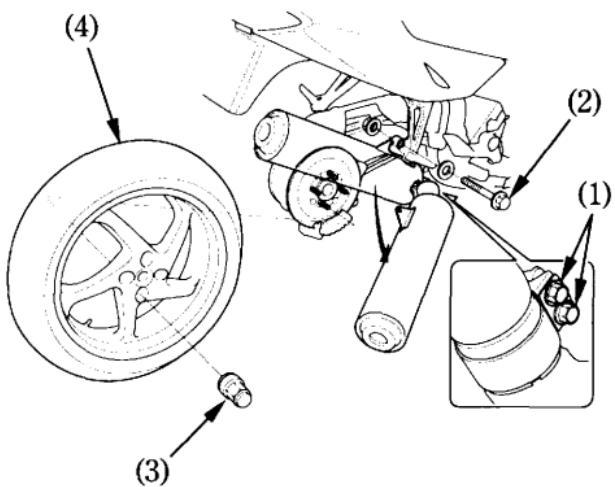
(1) Muffler clamp bolts      (3) Rear wheel nut
