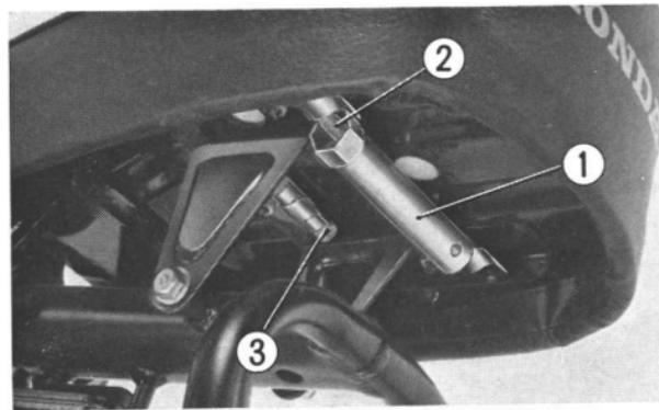
The spark plug wrench and valve joint are attached under the seat.
